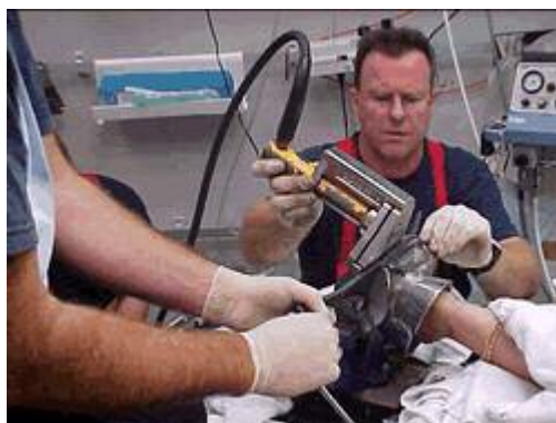
Jimmy bar being used to assist in splitting the casing of the mincer.
