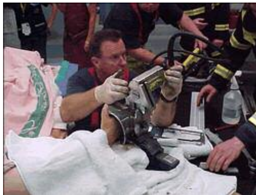
Rabbit tool being carefully applied after cuts to both sides of the casing and mounting plate.
