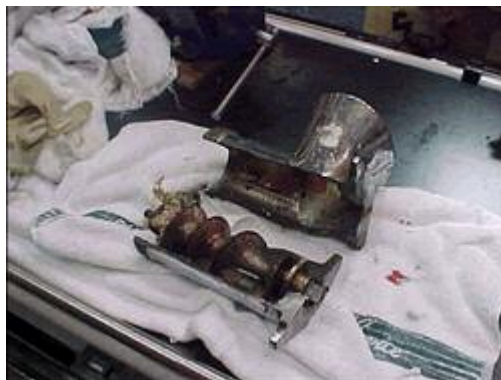
Cast iron casing revealing the auger and lower section.
